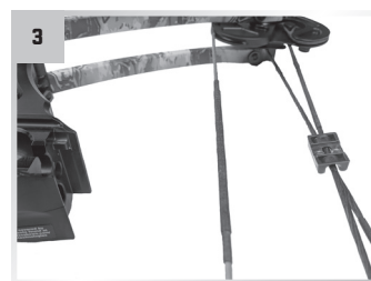
The mini-cross cable saver sits on top of the cables where they cross.
