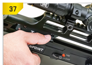
Press down on the forward assist knob.
