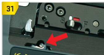
Trigger lock-latch hooked onto the trigger box pin.
