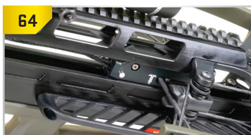
Trigger box attached to the bowstring.
