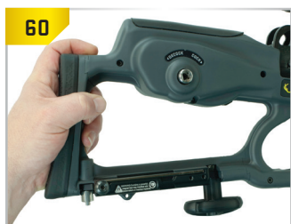
Insert the crank handle into its storage position in the stock.
