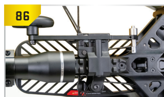
Mount to top of picatinny rail on left.
