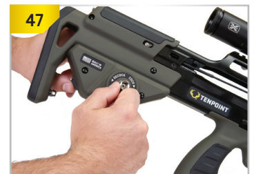
While holding the Gear Stop Button, back-wind the silver collar one (1) complete turn by hand or until it stops.
