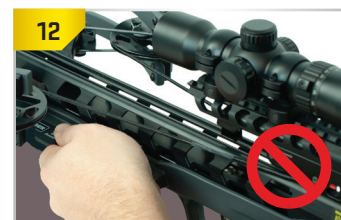
IMPROPER HAND POSITION. With your fore-grip hand positioned on top of the grip, you will severely injure or amputate your thumb and/or finger(s) if you fire your crossbow.
