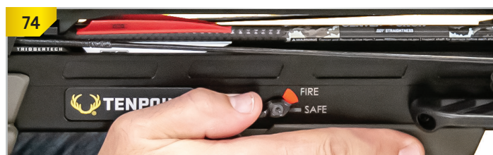
Slide the safety knob from SAFE (white) position to FIRE (red).
