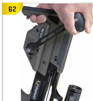
Press the trigger lock-latch down and backwind until the trigger moves 1/2-inch.
