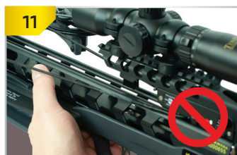
IMPROPER HAND POSITION. With your fore-grip rotated to the side of and/or above the grip/safety wings, you will expose your thumb to the bowstring's release path.
