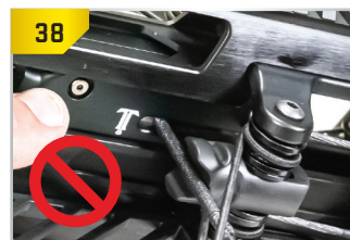
Improper string latch position.
