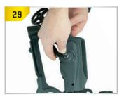
Insert crank handle into the ACUslide's square recess hole.
