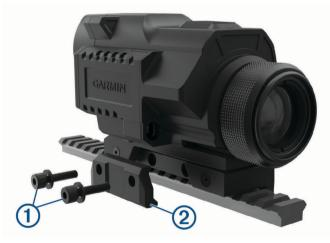
**3** Tighten the screws to a maximum torque specification of 2.5 N-m (22 lbf-in.).
