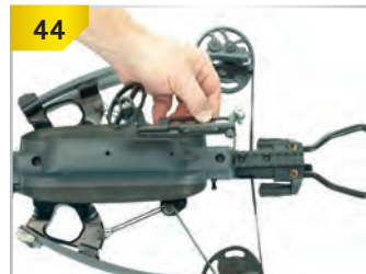
44 Push the trigger box release pin into the appropriate hole for your model.
