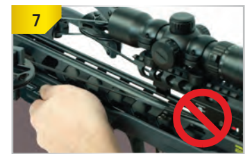
7 IMPROPER HAND POSITION. With your fore-grip hand positioned on top of the grip, you will severely injure or amputate your thumb and/or finger(s) if you fire your crossbow.
