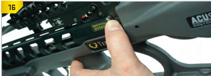
Press trigger box lock-latch lever.
