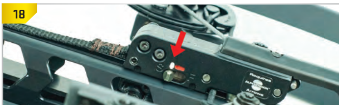
PROPER SAFETY POSITION. Safety knob in the "S" (Safe) position.
