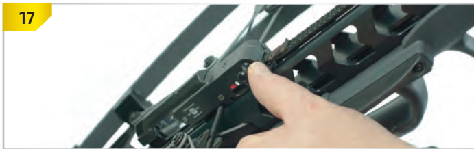
Push down on the forward assist knob.
