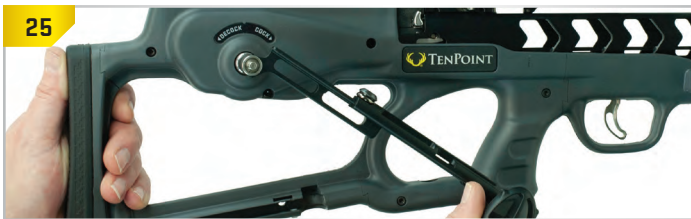
Backwind the crank handle two (2) complete turns.
