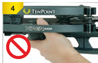
4 IMPROPER HAND POSITION. With your fore-grip hand positioned as shown, you will severely injure or amputate your thumb if you fire your crossbow.
