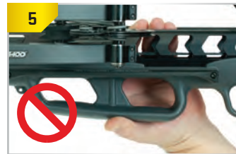
5 IMPROPER HAND POSITION. With your fore-grip hand positioned as shown, you will severely injure or amputate your thumb and/or finger(s) if you fire your crossbow.
