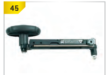
45 Slide the trigger release pin into the crank handle.
