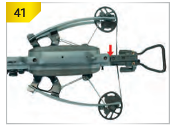
41 (2a) Release pin hole location on reverse-draw crossbows.
