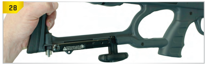
Insert the crank handle into its storage position in the stock.
