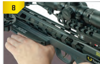
6 IMPROPER HAND POSITION. With your fore-grip rotated to the side of and/or above the grip/safety wings, you will expose your thumb to the bowstring's release path.
