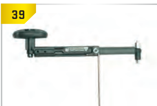
39 Extend trigger box release pin.
