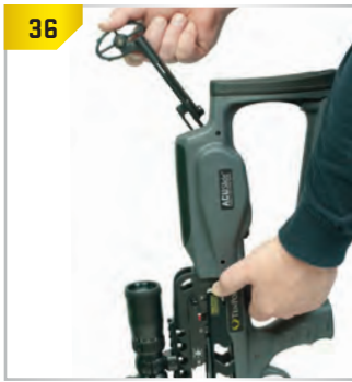
36 Hold the trigger lock-latch lever down and backwind until the trigger box moves 1/2-inch.
