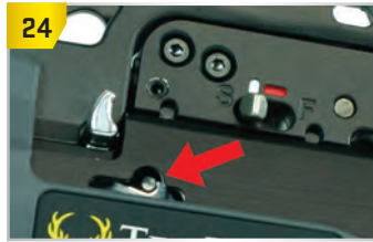
Trigger lock-latch hooked onto the trigger box pin.
