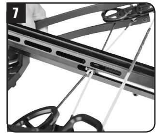
Tilt riser and slide it out of the barrel.
