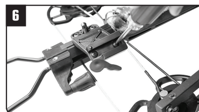
Install the quick disconnect (female) attachment.
