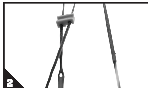
Make certain your cables go into the correct slots in your cable saver.
