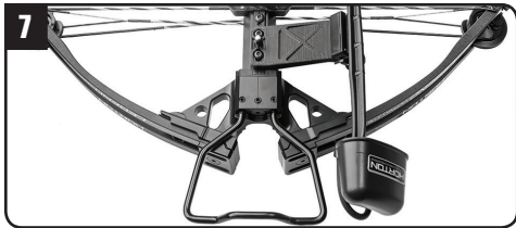
Insert the 3-Arrow Instant Detach Quiver into the female bracket and lock into place with the lever.
