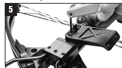
Place the quiver bracket assembly over the two barrel holes and insert 3/4" screws.
