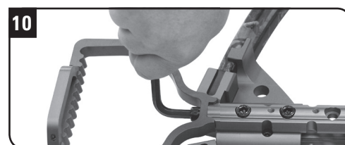
Attach the foot stirrup directly to the bottom section of the UL TriLoc barrel. See page 3 if mounting the 3-Arrow Instant Detach Quiver.
