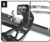
Remove screws from the bottom of the riser.
