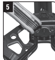
Place the quiver bracket assembly over the two setscrew holes and insert 3/4-inch setscrews and Nylock nuts.
