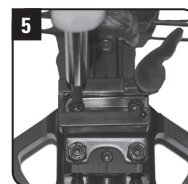
Install the quick disconnect (female) attachment.
