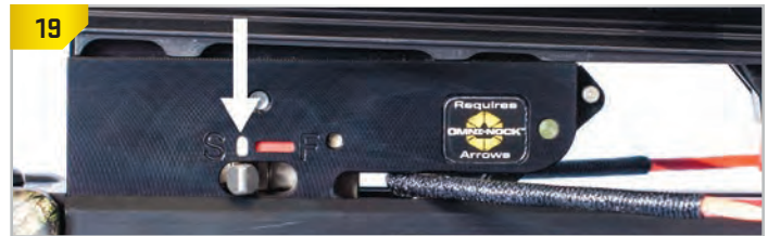
When you cock your crossbow correctly, the safety will automatically move to the SAFE (white) position, and the string latch will engage the string.
