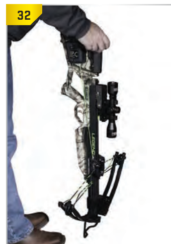
Engage the safety pawl, insert the crank and begin cranking.
