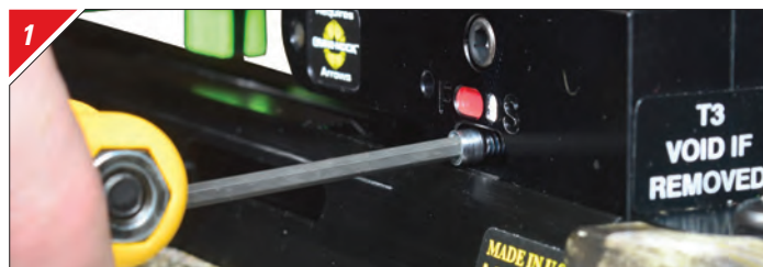
Remove the hex-head cap screw.
