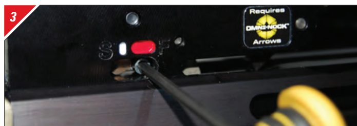
Re-insert the hex-head cap screw into the safety knob.
