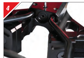
Loosen locking setscrew before turning the main assembly bolt.
