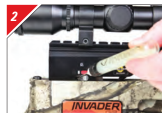
Lubricate the trigger through the safety slide window.
