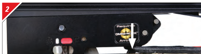
If you try to cock the crossbow while the safety is in the SAFE position (rearward, toward the white dot), the DFI will hold the bowstring and the bow will only appear to be cocked.
