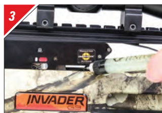
Apply a drop just inside the closed end of the trigger's string slot.
