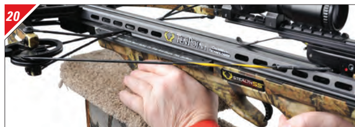
Keep your thumb and fingers below the flight deck and away from the cables to avoid injury.
