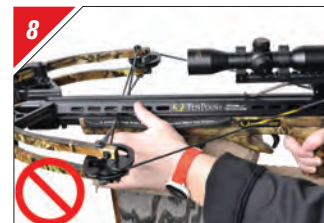
8 IMPROPER POSITION. With your fore-grip hand rotated to the side of the grip, you will expose your thumb to the bowstring's release path.
