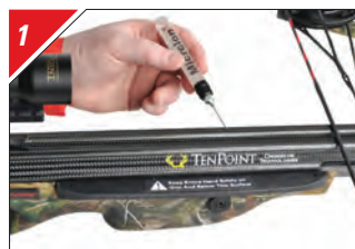
Lubricate your flight rail approximately every 75 to 100 shots with flight rail lubricant or 150 to 200 shots with Microlon's® Precision Oiler.
