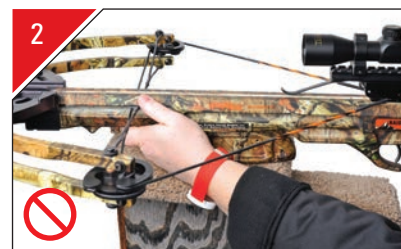
IMPROPER POSITION. With your fore-grip hand positioned in front of the grip, you will expose your thumb to the bowstring's release path.
