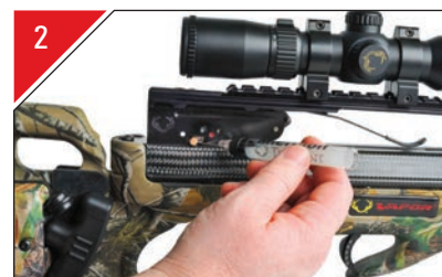
Lubricate the PowerTouch Trigger through the safety slide window.
