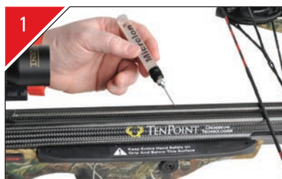
Lubricate your flight rail approximately every 75 to 100 shots with flight rail lubricant or 150 to 200 shots with Microlon's® Precision Oiler.
