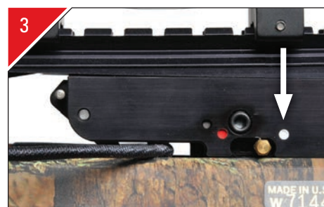
When you cock your crossbow correctly, the safety will automatically move to the SAFE position (rearward, toward the white dot), and the string latch will engage the string.
