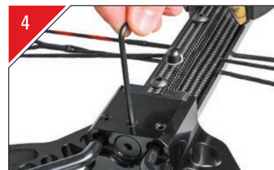
Loosen locking setscrews before turning the main assembly bolt or limb bolts (limb bolt locking setscrews only on certain older-series TenPoint Series crossbow models).
