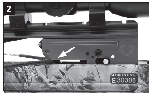
If you try to cock the crossbow while the safety is in the rear, SAFE (white dot) position, the bow-string will be held by the DFI™ and only appear to be cocked.
