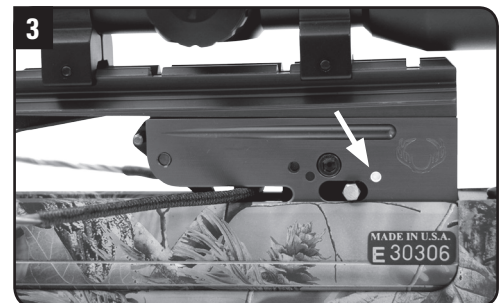
When you cock your crossbow correctly, the safety will automatically move to the rear, SAFE (white dot) position, and the string latch will engage the string.
