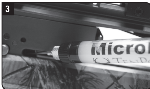
Apply a drop just inside the closed end of the trigger's string slot.
