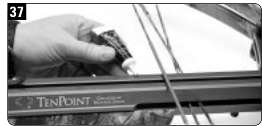
Lubricate your flight rail approximately every 75 to 100 shots with flight rail lubricant or 150 to 200 shots with Microlon's Precision Oiler.
