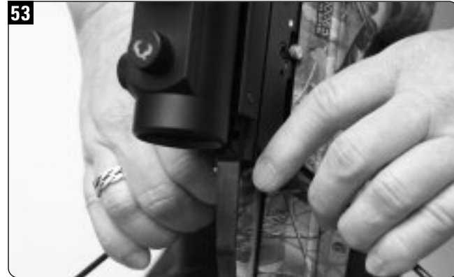
Push the DFI pin down with the index finger.
