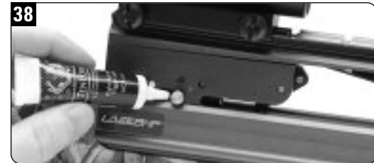
Lubricate the Power Touch Trigger through the safety slide window.
