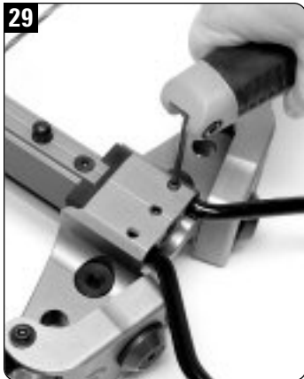
Remove 1/4-inch setscrews from the bottom of the riser (not applicable to CLS models).
