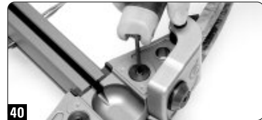
Loosen locking setscrews before turning the main assembly bolt or limb bolts (on certain TenPoint Series crossbow models).
