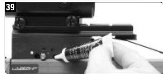
Apply a drop just inside the closed end of the trigger's string slot.
