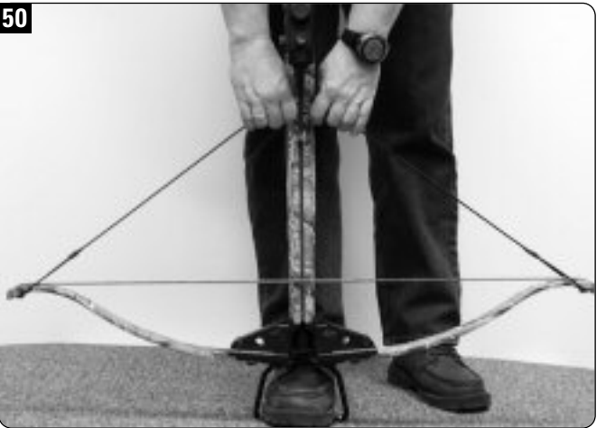
Pull the re-stringer back toward the trigger box until the re-stringer is sitting on the dry-fire inhibitor.
