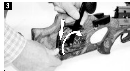
Properly relieve the tension on the ACUdraw unit before lifting the claw out of its storage position (approximately 1/4-inch to 1/2-inch).
