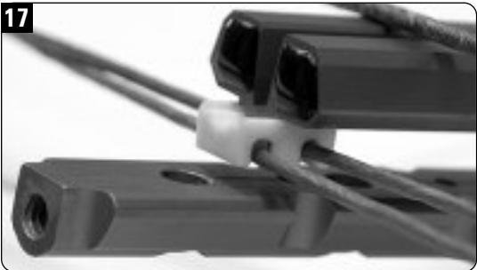
The cable saver's concave groove ("dish") should mate with the underside of the barrel's arrow flight groove (cable saver and cables not applicable to the GT Mag or GT Flex).
