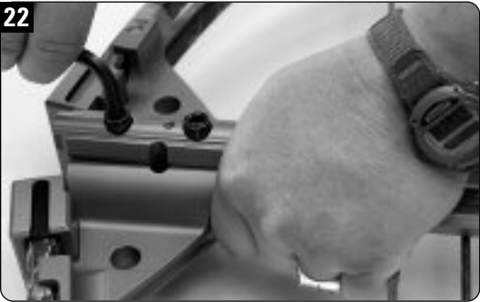
Squeeze the top and bottom of the barrel with your free hand when tightening the two large bow assembly bolts.
