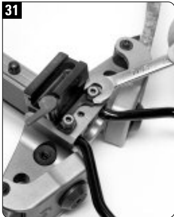
Tighten the Nylock nuts with a 7/16-inch open-ended wrench.
