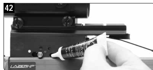
Apply a drop just inside the closed end of the trigger's string slot.
