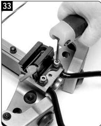
Place the quiver bracket assembly over the two setscrew holes and insert 3/4-inch setscrews with Nylock nuts.
