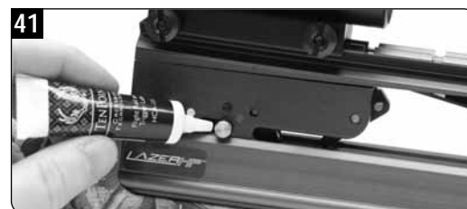
Lubricate the Power Touch Trigger through the safety slide window.
