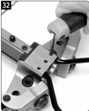
Remove 1/4-inch setscrews from the bottom of the riser.
