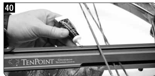
Lubricate your flight rail approximately every 75 to 100 shots with flight rail lubricant or 150 to 200 shots with Microton's Precision Oiler.
