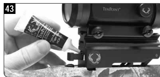
Lubricate the RollerTouch safety plunger shaft.
