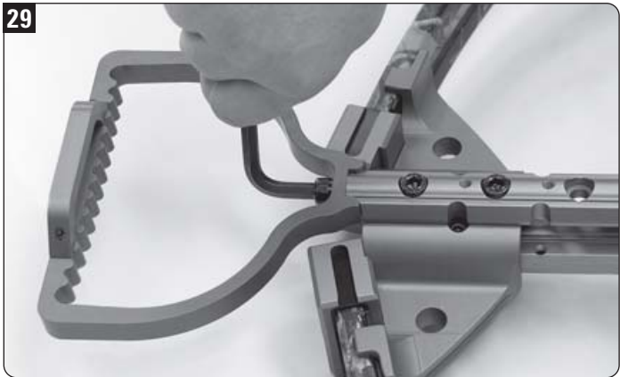
Attach the foot stirrup directly to the bottom section of the UL TriLoc barrel. See page 14 if mounting the HX Instant Detach Quiver.
