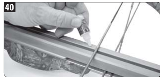
Lubricate your flight rail approximately every 75 to 100 shots with flight rail lubricant or 150-200 shots with Microlon's Precision Oiler.
