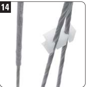
Make certain your cables go in the correct slots in your cable saver.
