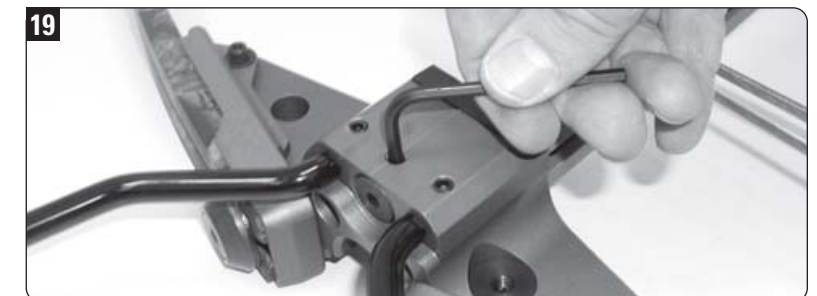
Once the foot stirrup is in place, tighten all three locking setscrews (foot stirrup setscrews not applicable to the Phantom CLS). See page 13 if mounting the HX Instant Detach Quiver.
