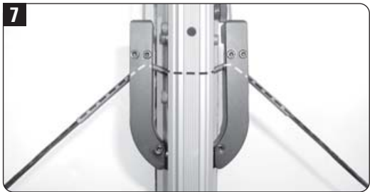
Notice that the string is under heavy tension once the bow is cocked.
