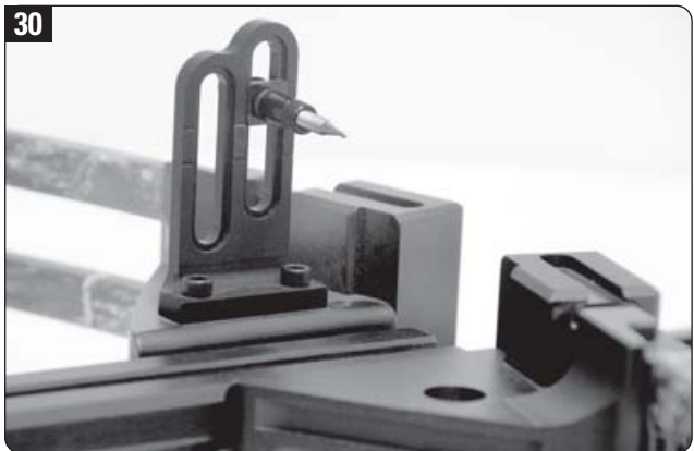
Mount your front sight on the left-hand side of the riser (Titan TL-7 and Slider models).
