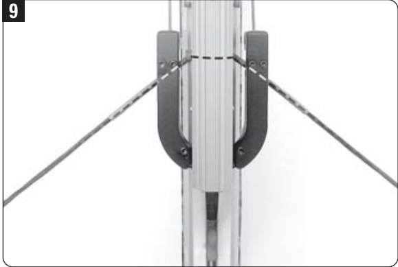
After 2 1/2 to 3 reverse turns you can see and feel that the pressure is off the claw. You can then remove the crank.
