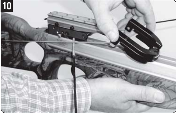
Once you relieve the string tension on your cocked crossbow, remove the crank so you can slide the claw forward.
