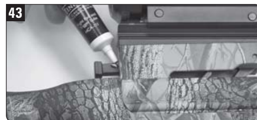
Lubricate the RollerTouch safety plunger shaft.
