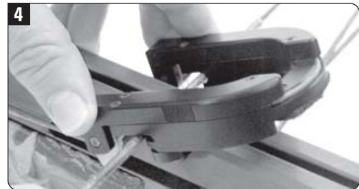
Connect the string slots to the bowstring and lower the guidepost into the barrel's flight groove.
