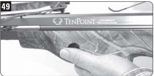
Depress the GripSafety with your thumb before squeezing the trigger.
