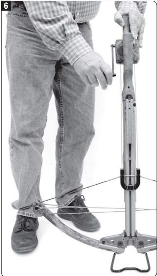
Engage the safety pawl, insert the crank, and begin cranking.
