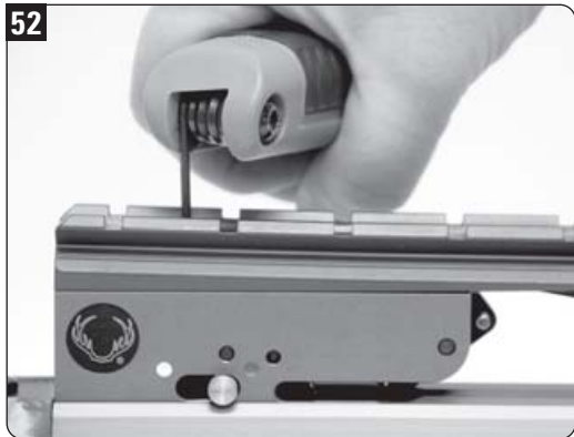
Access the safety tension screw through the top of the dovetail on PowerTouch trigger boxes. Access the safety tension screw through the top of the sight bridge on RollerTouch trigger boxes.
