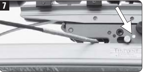
When you cock your crossbow correctly, the safety will automatically move to the rear, SAFE (white dot) position, and the string latch will engage the string.
