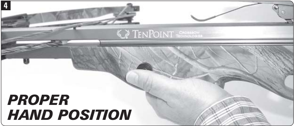
Proper way to hold the fore-grip. Note the GripSafety™ button located on the side of the fore-grip. Refer to page 15 for details.
