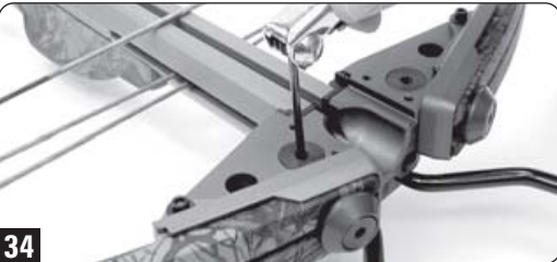
Loosen locking setscrews before turning limb bolts or the main assembly bolt (on TenPoint Series crossbows).
