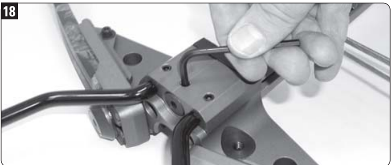
Once the foot stirrup is in place, tighten all three locking setscrews.
