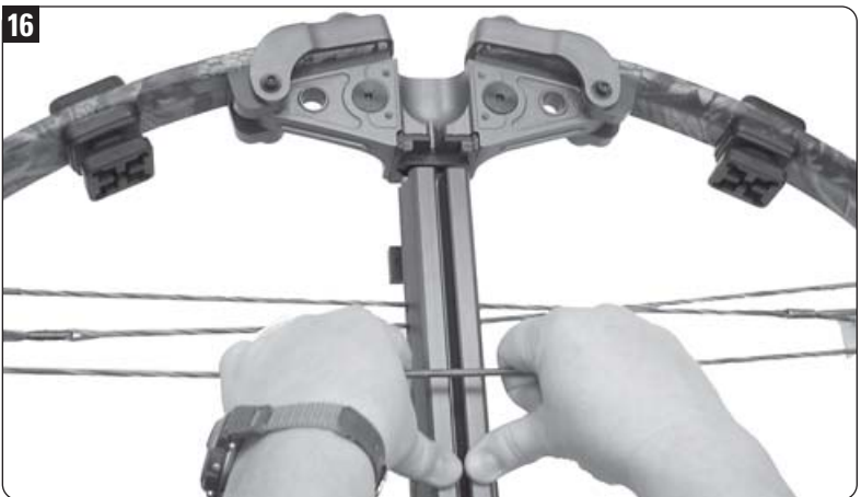
Pull up and back slightly on the bow string to seat the bow assembly.
