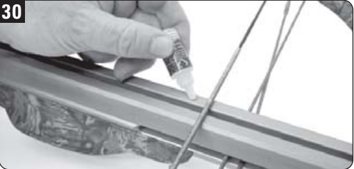
Lubricate your flight rail approximately every 75 to 100 shots.
