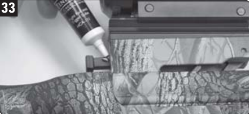
Lubricate the RollerTouch or DropLatch safety plunger shaft.
