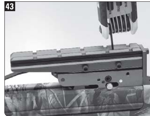
Access the safety tension screw through the top of the dovetail on PowerTouch trigger boxes. Access the safety tension screw through the top of the sight bridge on RollerTouch or DropLatch trigger boxes.
