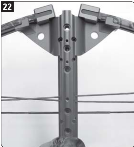
Bow assembly in “long” position.
