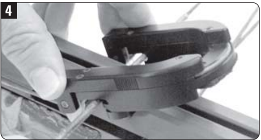
Connect the string slots to the bowstring and lower the guidepost into the barrel's flight groove.
