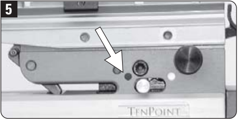
Make sure the trigger's safety is in the forward, FIRE (red dot) position before cocking your crossbow.
