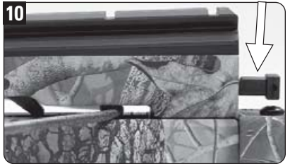
When you cock your crossbow correctly, the safety will automatically move to the rear, SAFE (white dot) position, and the string latch will engage the string.
