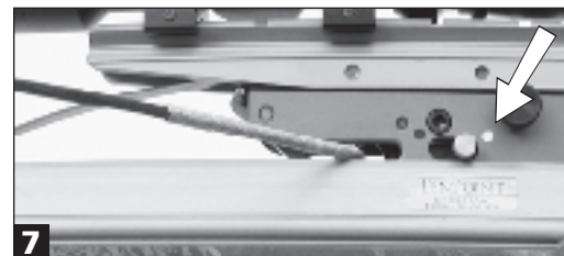
7 When you cock your crossbow correctly, the safety will automatically move to SAFE (white dot) and the string latch will engage the string.
