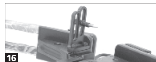
You can mount your front sight on either side of the riser.
