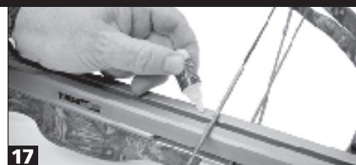
17 Lubricate your flight rail approximately every 75 to 100 shots.
