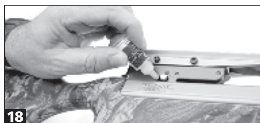
18 Lubricate the PowerTouch trigger through the safety slide window.
