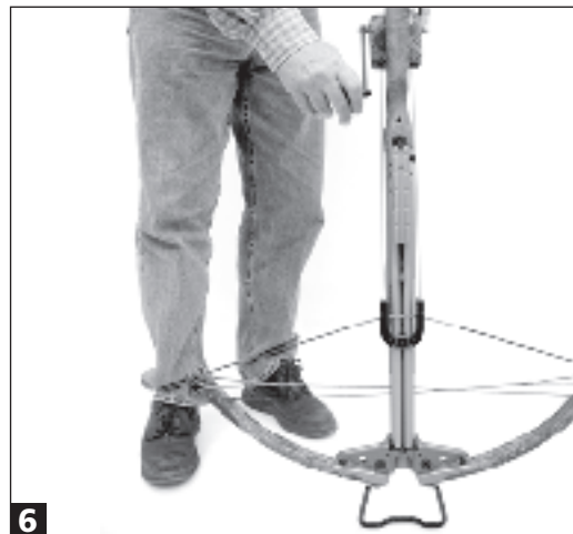
6 Engage the safety pawl, insert the crank, and begin cranking.
