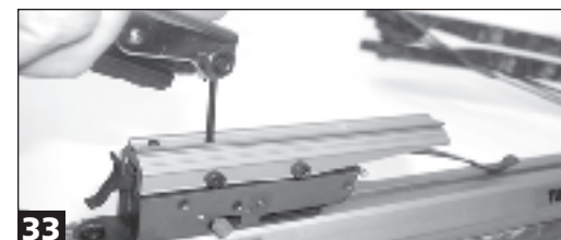
Access the safety tension screw through the top of the dovetail on ELITE or QX-4 Series models. Access the safety tension screw through the top of the sight bridge on HYBRID LITE or TITAN TL-4 models.
