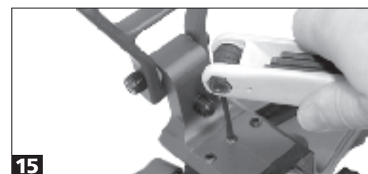
Once the drop-tine stirrup is in place, tighten the main assembly bolt setscrew.
