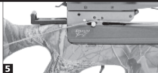
5 Don't allow the draw cord to get hung-up on any part of the crossbow, scope or accessories.
