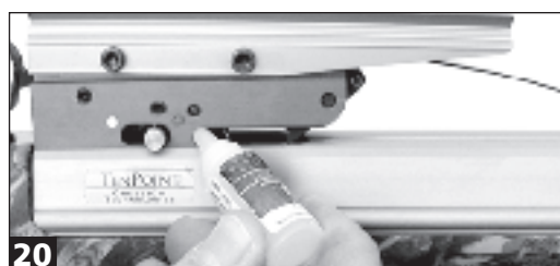
20 Apply a drop just inside the closed end of the trigger's string slot.
