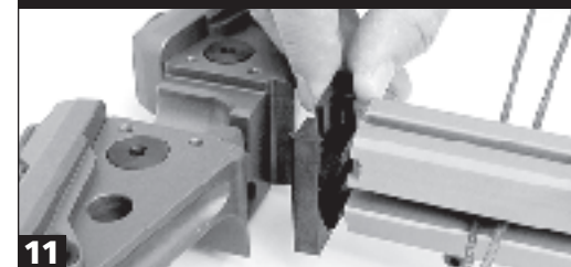
The VIBRA-CUSH goes between the riser and the barrel, cutout side facing the barrel.
