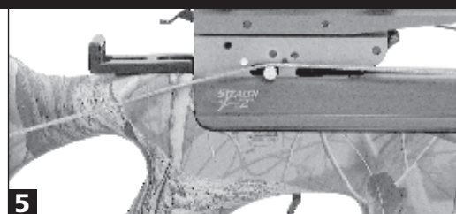
5 Don't allow the draw cord to get hung-up on any part of the crossbow or accessories.
