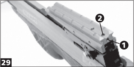
29 Loosen the locking setscrew (1) before setting the dovetail pitch-adjustment screw (2).
