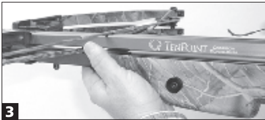
With your foregrip hand positioned near the crossbow cables as shown above, you will severely injure your fingers if you fire your crossbow.
