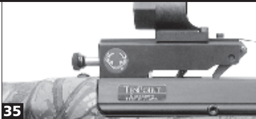
35 The TITAN™ trigger has an ambidextrous plunger safety and a drop or down latch bowstring catch. The safety is shown in the SAFE position in this photo.
