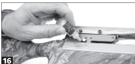
16 Lubricate the PowerTouch trigger through the safety slide window.
