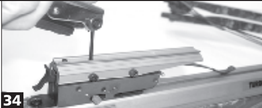
34 Access the safety tension screw through the top of the dovetail on X-2 Series models. Access the safety tension screw through the top of the sight bridge on TITAN® models.
