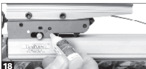
18 Apply a drop just inside the closed end of trigger's string slot.
