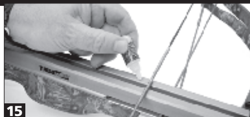
15 Lubricate your flight rails every 40 to 50 shots.
