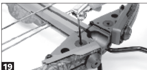
19 Loosen locking set screws before turning limb bolts or the main assembly bolt.
