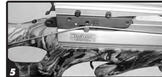
Don't allow the draw cord to get hung-up on any part of the bow.
