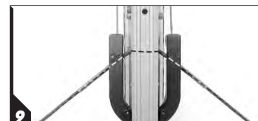
After three reverse turns you can see that the pressure is off the claw. You can then remove the crank.
