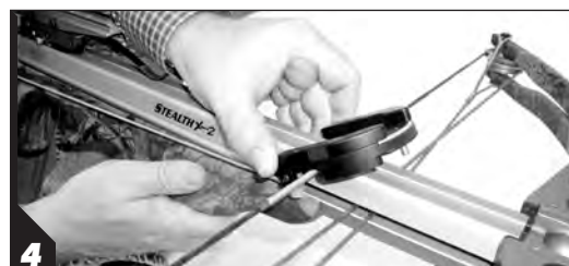
Connect the string slots to the bowstring and lower the guidepost into the barrel's flight groove.
