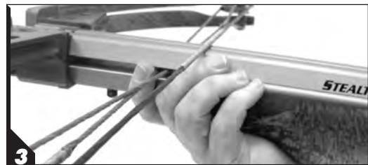
3 With your foregrip hand positioned near the crossbow cables as shown above, you will severely injure your fingers if you fire your crossbow.
