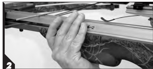
2 With your foregrip hand positioned as shown above, you will severely injure your fingers when you fire your crossbow.
