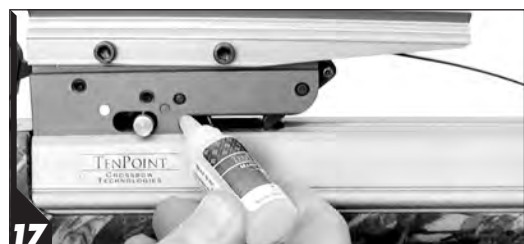
17 Apply a drop just inside the closed end of trigger's string slot
