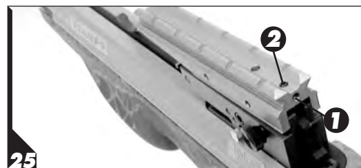
25 Loosen the locking setscrew (1) before setting the dovetail pitch-adjustment screw (2).
