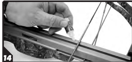
14 Lubricate your flight rails every 40 to 50 shots.
