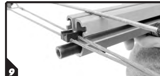
The bow string rests on the barrel's flight deck while the cable saver and cables slide into the cable slot.
