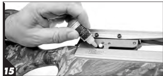
15 Lubricate the PowerTouch trigger through the safety slide window.
