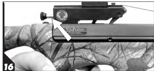
16 Lubricate the TITAN's safety plunger shaft
