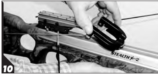
10 Once you relieve the sting tension on your cocked crossbow and remove the crank, you can slide the claw forward and return it to its storage position.
