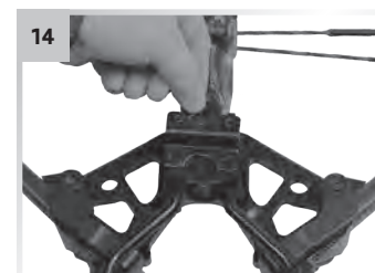
Place the quiver mount bracket over the two foot stirrup setscrew holes.
