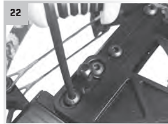
22 Insert and tighten two 1/4-20 x 3/4-inch button-head cap screws.
