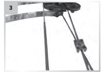
The mini-cross cable saver sits on top of the cables where they cross.
