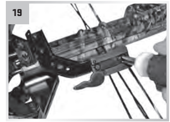
19 Install the female lever-lock attachment.
