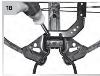
18 Attach the side-mount bracket to the quiver mounting bracket assembly.
