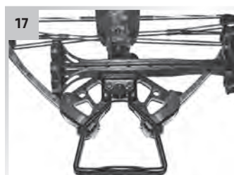
Insert the 3/4-inch setscrews & Nylock nuts (use the 1-inch setscrews for Wicked Ridge crossbows).
