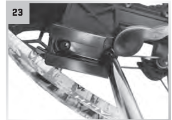
23 Install the quick disconnect (female) attachment.
