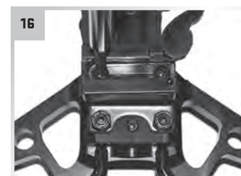
Install the quick disconnect (female) attachment.
