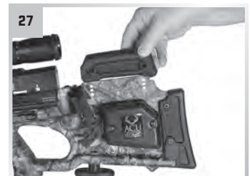
27 Slide cheek piece over desired alignment holes.
