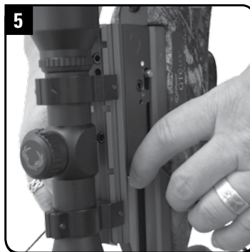
Push the DFI pin down with the index finger.
