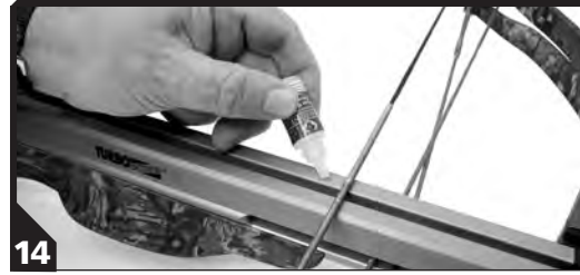
14 Lubricate your flight rails every 40 to 50 shots.
