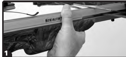
1 With your foregrip hand positioned as shown above, you will severely injure your thumb if you fire your crossbow.
