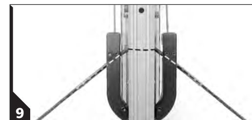
9 After three reverse turns you can see that the pressure is off the claw. You can then remove the crank.
