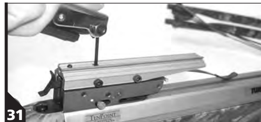
31 Access the safety tension screw through the top of the dovetail on STEALTH™, MAGNUM™, and TURBO™ models. Access the safety tension screw through the top of the sight bridge on WoodsMan™ and TITAN™ models.
