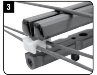
The cable saver's concave groove ("dish") should mate with the underside of the barrel's arrow flight groove.
