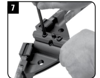
Continue to squeeze the top and bottom of the barrel with your free hand when tightening the two larger bow assembly bolts.
