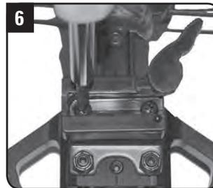
Install the quick disconnect (female) attachment.
