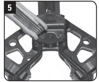
Place the quiver bracket assembly over the two setscrew holes and insert 3/4-inch setscrew and Nylock nuts.
