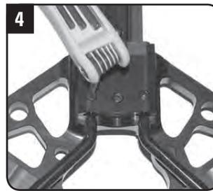
Remove 1/4-inch setscrews holding foot stirrup in place.
