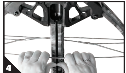
4 Pull up and back slightly on the bow string to seat the bow assembly.
