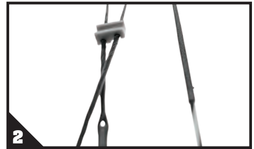
2 Make certain your cables go into the correct slots in your cable saver.
