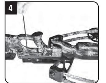
Install rear stock screw and partially tighten.
