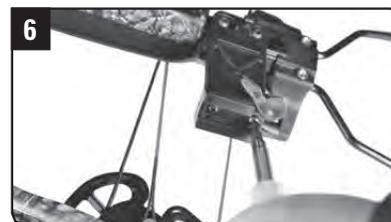
Install the quick disconnect (female) attachment.
