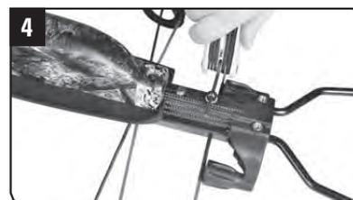
Remove sling stud and  $\frac{3}{8}$ " barrel screw.
