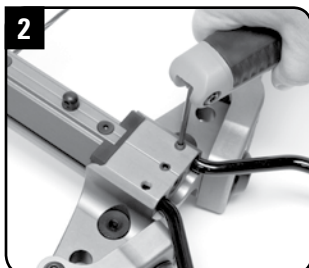
Remove 1/4-inch setscrews from the bottom of the riser.
