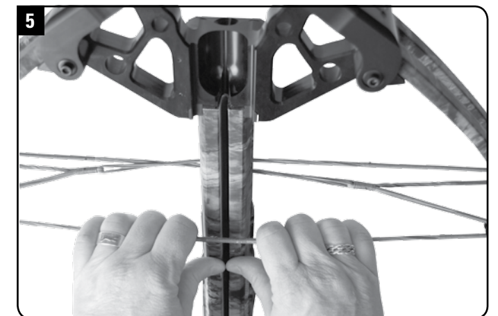
Pull up and back slightly on the bow string to seat the bow assembly.
