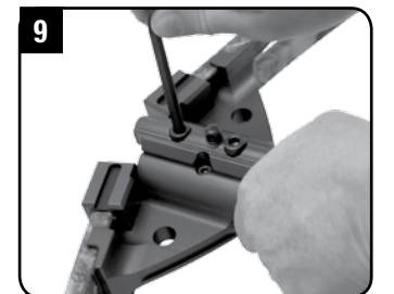
Continue to squeeze the top and bottom of the barrel with your free hand when tightening the two larger bow assembly bolts.
