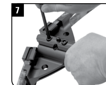
Continue to squeeze the top and bottom of the barrel with your free hand when tightening the two larger bow assembly bolts.
