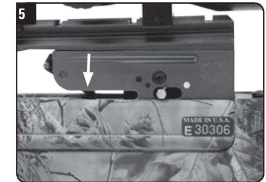
TenPoint's patented DFI™ (Dry-Fire Inhibitor).
