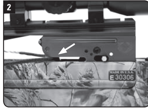
If you try to cock the crossbow while the safety is in the rear, SAFE (white dot) position, the bowstring will be held by the DFI™ and only appear to be cocked.
