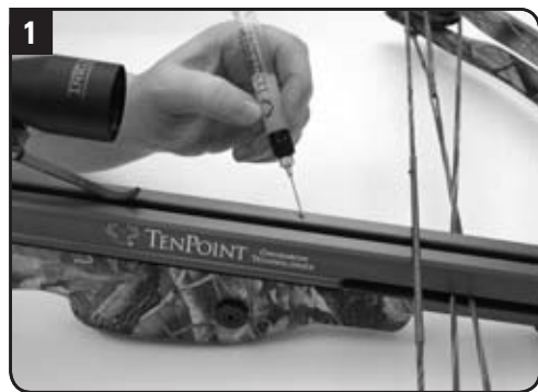
Lubricate your flight rail approximately every 75 to 100 shots with flight rail lubricant or 150 to 200 shots with Microlon's Precision Oiler.
