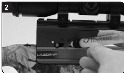
Lubricate the PowerTouch Trigger through the safety slide window.
