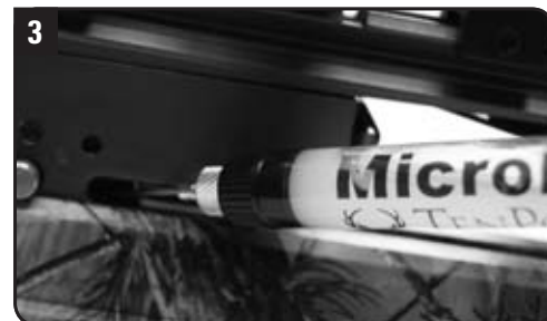
Apply a drop just inside the closed end of the trigger's string slot.
