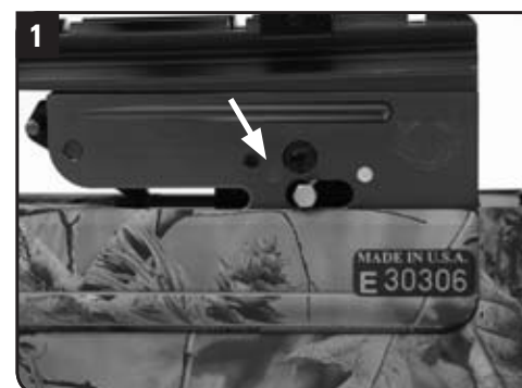
Make sure the trigger's safety is in the forward, FIRE (red dot) position before cocking your crossbow.
